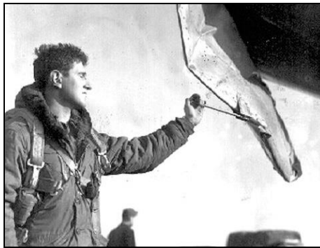
2 ND LT. LAURENCE J. LAZZARI INSPECTING MID-AIR COLLISION DAMAGE
