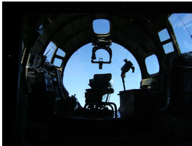
LOOKING OUT FRONT BLISTER TO BOMBARDIER/TOGGLEIER POSITION FROM RESTORED B-17 RE-NAMED 'NINE-O-NINE' - WINGS OF FREEDOM TOUR
